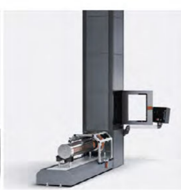
Rapid Crack Propagation RCP
