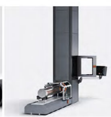
Rapid Crack Propagation RCP
