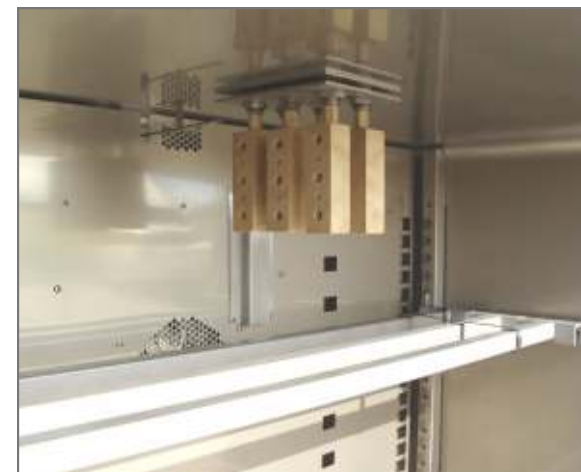
View inside heating oven - optional manifolds (access ports) for connecting pipe samples in case connection to pressure testing equipment is needed. Further, the optional sample hanging bars are shown (three pieces in picture above) for hanging pipe samples.
