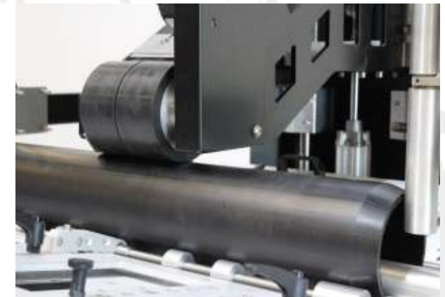
Pipe rotater with automatic centering
