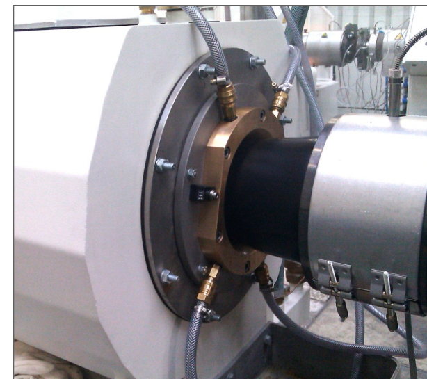
An installed calibrating sleeve in action ensuring close-to-minimum-tolerance production and a reduction of overall scrap volume.
